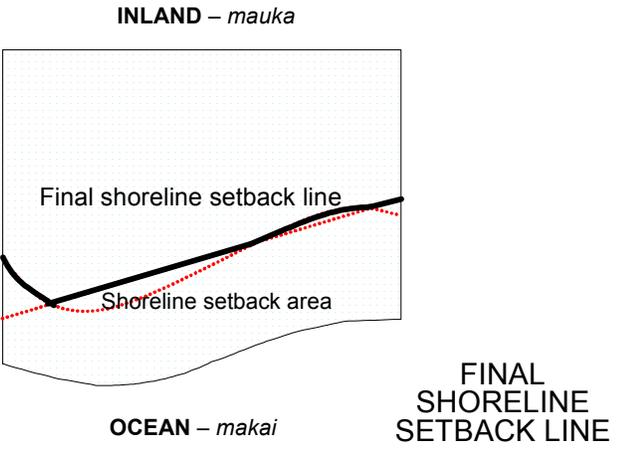
10. The site plan should illustrate both the lot-depth based setback (ALD) and the erosion-rate based setback (AEHR), as well as their calculations (Figure 3). The more mauka (inland) of the lines forms the shoreline setback line. In the unusual circumstance that the lines cross each other, the more mauka segments of each line form the shoreline setback line (Figure 4).
