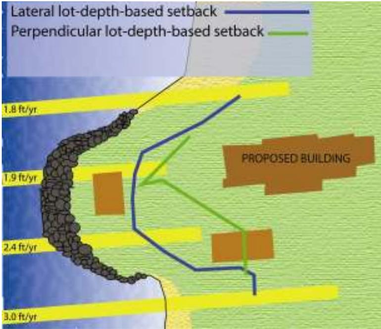
9. Calculate the Shoreline Setback Line (SSL) based on the erosion rate for the site, if and where applicable. See Figure 2. Erosion rates are established for most sections of the South, North and West shoreline areas on the island of Maui.
